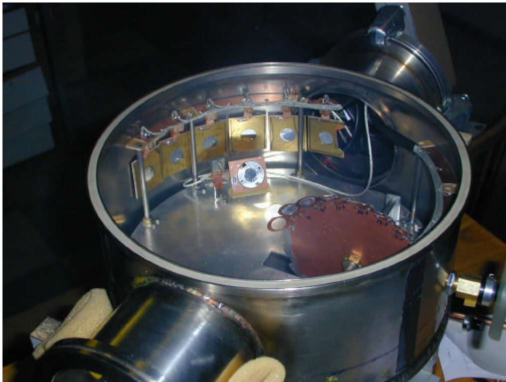
Fig. 2-3. The general view of the reaction vacuum chamber.
